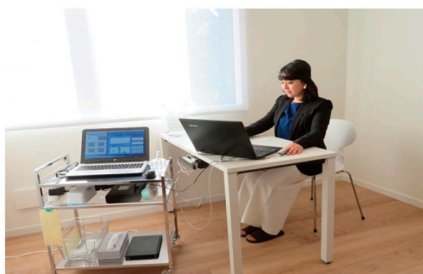
Figure 3. Subject attaches the probe to its head. After starting the EEG measurement, they begin to perform the tasks of calculation, memorization, and rest, according to the PC navigation.
