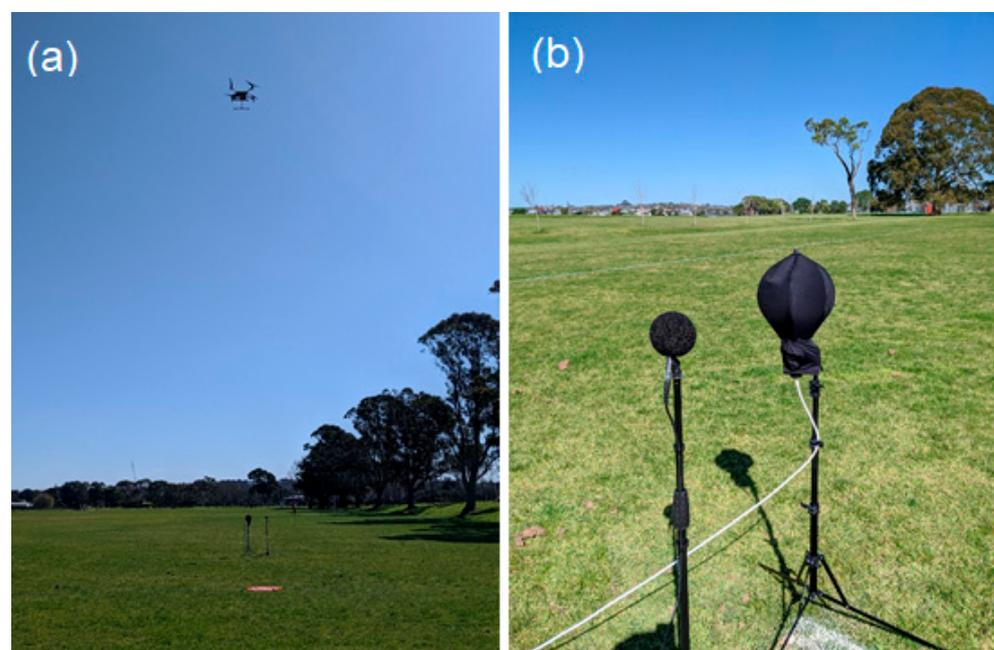
**Figure 2.** (a) The Matrice quadcopter UAV hovering above the two microphones; (b) the 1/2" microphone and Eigenmike with wind socks mounted on tripods.
