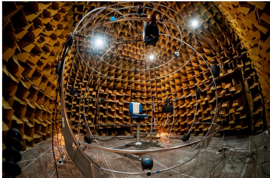
**Figure 3.** Sixteen-channel spherical loudspeaker array setup in the anechoic chamber at the University of Auckland (taken from [51]).
