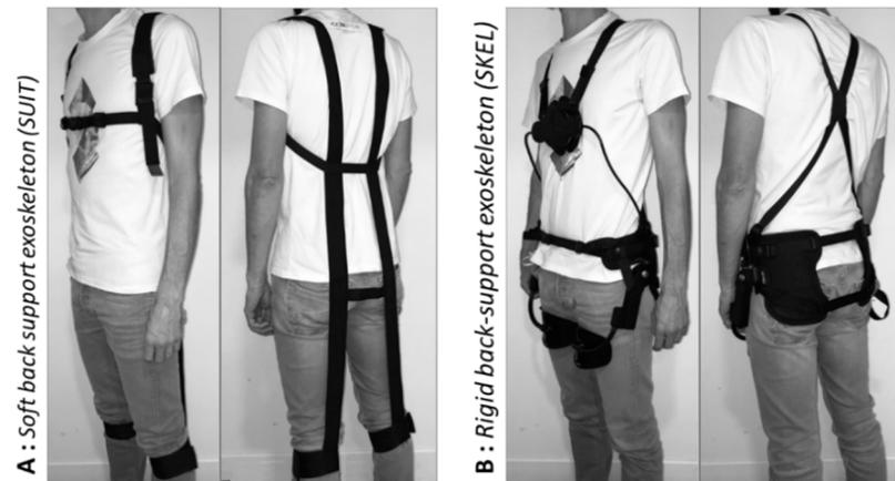
**Figure 2.** The two exoskeletons used; (A) soft back-support exoskeleton or exosuit (SUIT) (Corfor<sup>®</sup>-V2, Villemus, France), and (B) rigid back-support exoskeleton (SKEL) (Laevo<sup>®</sup>-V1, Deft, The Netherlands).
