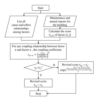
Figure 6. The flow chart of our coupling revision algorithm.
