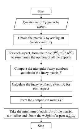
Figure 4. The flow chart of the FAHP algorithm.
