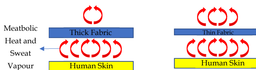
Figure 6. Heat transfer through thick and thin fabrics for THL.
