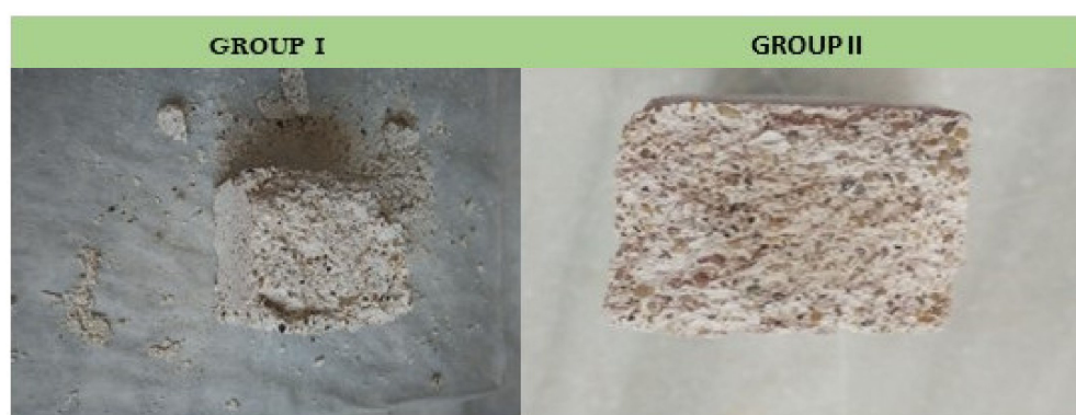
Figure 11. View of the fracture of representative specimens of Group Ia and IIa after 21 days in environmental chamber.
