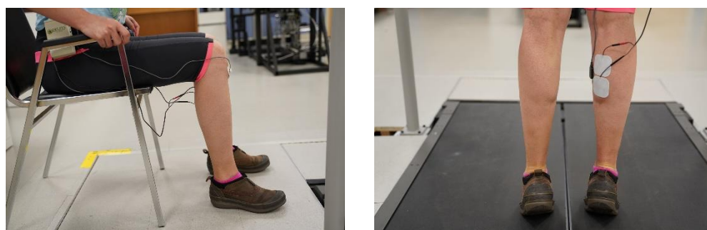
Figure 2. (Left): Drift test—participants spent 5 min in a seated position with knees flexed at 90 degrees and were instructed not to move. (Right): Lag test—participants performed heel rises to match a metronome at 45, 60, 75, and 90 BPM for 30 s.
