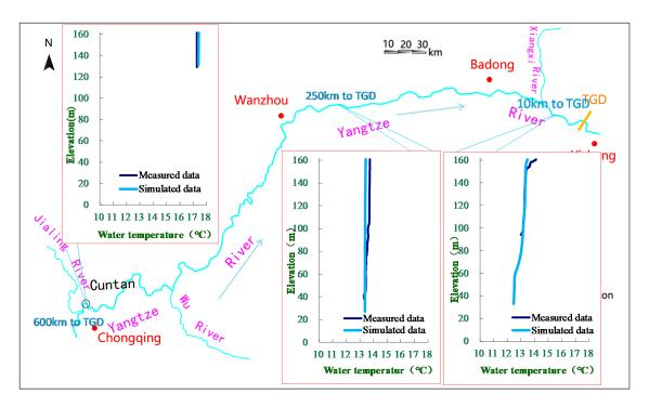
Figure 3. Comparison of simulated and measured water temperatures in the Three Gorges Reservoir on 28 March 2013.
