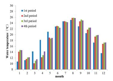
Figure 8. Monthly discharge water temperature of the Three Gorges dam.
