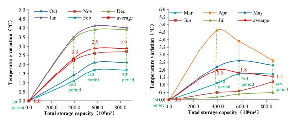
**Figure 9.** The difference between the discharged water temperature of the TGD and the natural water temperature. The total storage capacity is the sum of the storage capacity of each reservoir. In the 1st period, the total storage capacity is 0. In the 2nd period, the total storage capacity is  $393 \times 10^8$  m<sup>3</sup>. In the 3rd period, the total storage capacity is  $574 \times 10^8$  m<sup>3</sup>. In the 4th period, the total storage capacity is  $853 \times 10^8$  m<sup>3</sup>.
