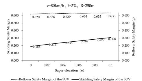
**Figure 10.** Skidding and rollover safety margin of the SUV on poor friction pavement ( $f_{Tmax} = 0.50$ ) (Case 1–6, in Table 5).
