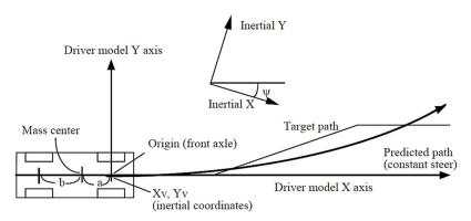
Figure 3. Axis system of steering controller.
