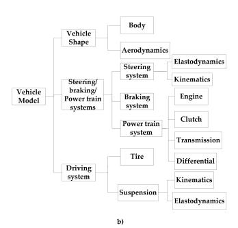
Figure 2. (a) 27-Degree of Freedom (DOF) Vehicle Model. (b) CarSim Vehicle Structure.
