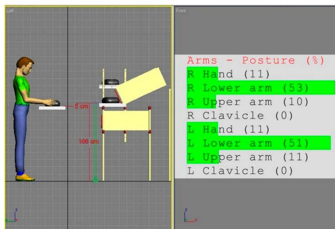
**Figure 4.** Simulation of modified workstation (a) adjusted to the optimal hand configuration of the 50th percentile mannequin of the Eastern European population. This arrangement's risk score for Part B of the REBA method is minimal.
