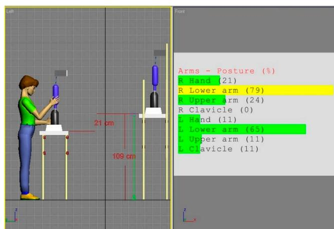
**Figure 10.** Simulation of 5th percentile woman on the modified workstation (b) adjusted to the optimal hand configuration of the 50th percentile individual.
