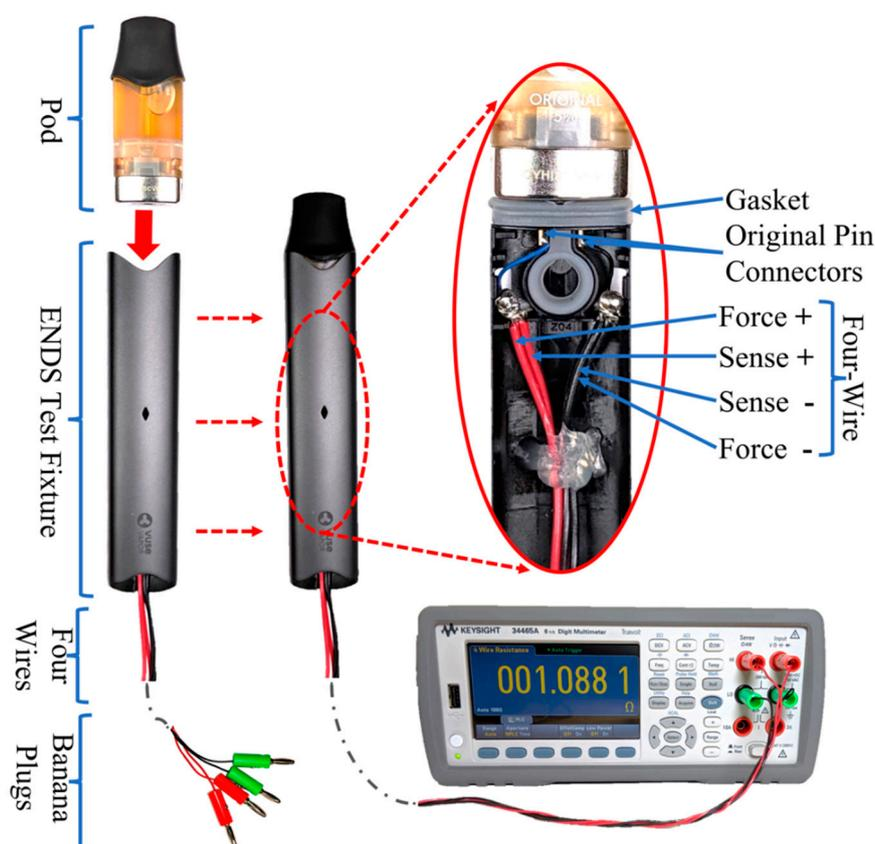
**Figure 3.** Custom electronic nicotine delivery systems (ENDS) test fixture for Vuse/ALTO pod-style ENDS coil resistance measurement in conjunction with a Keysight Model 34465A digital multimeter. The exploded view shows an inside view of the wire connections.
