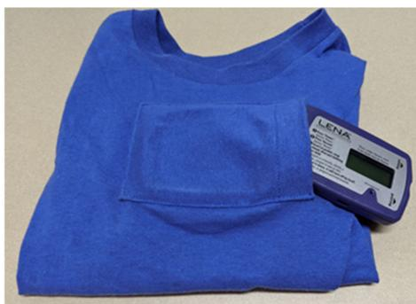
**Figure 4.** The Language Environment Analysis System (LENA Research Foundation, 2015) alongside the specially made t-shirt. The chest pocket secures the LENA throughout the day with a snap button.
