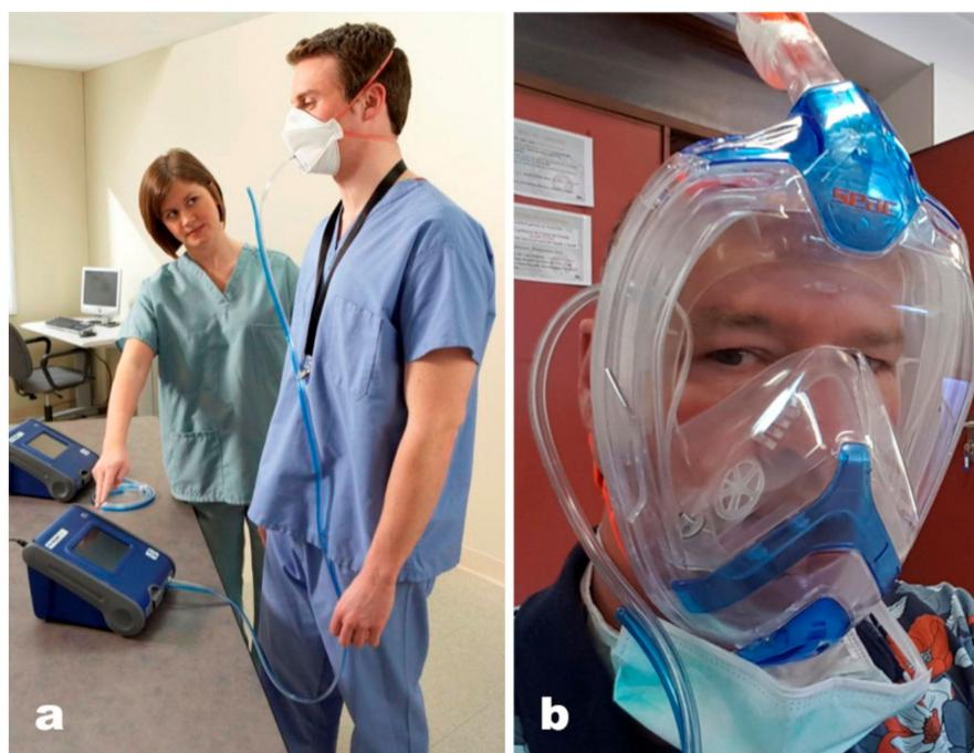
**Figure 3.** Particle count sampling setup. (a) (from [12]) general setup; (b) sampling tube fitted inside snorkel mask towards nose and mouth breathing chamber. Blue tubing—ambient air sampling line, transparent tubing—mask sampling line.
