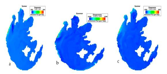
Figure 6. (a) 11th, (b) 41st, (c) 70th day simulation of NH<sub>4</sub> flux variation during summer at Taihu.
