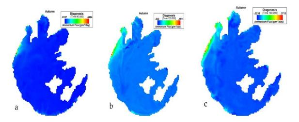
Figure 7. (a) 90th, (b) 120th, (c) 140th day simulation of NH<sub>4</sub> flux variation during autumn at Taihu.
