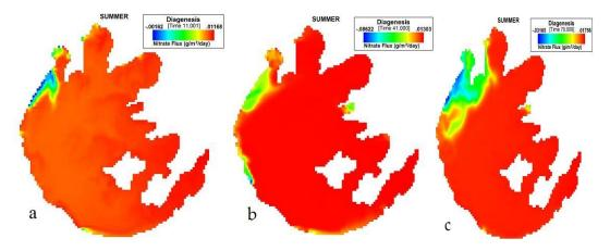
Figure 2. (a) 11th, (b) 41st, (c) 70th day simulation of NO<sub>3</sub> flux variation during summer at Taihu.
