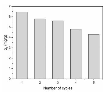
**Figure 15.** Reusability of BiFeO<sub>3</sub>/biochar coupled magnetic material for methylene blue removal (V = 0.05 L, T = 25 °C, t = 240 min, pH=6, m = 0.1299 g).
