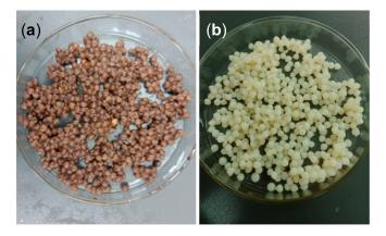
Figure 1. BiFeO<sub>3</sub>/biochar coupled magnetic beads (a) and blank beads (b).
