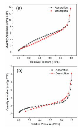
Figure 4. Nitrogen adsorption-desorption isotherms of (a) BiFeO<sub>3</sub> and (b) BiFeO<sub>3</sub>/biochar.
