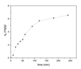
**Figure 12.** Effect of reaction time on the adsorption process (V = 0.15 L, pH = 6.0, T = 25 °C, m = 0.3889 g).
