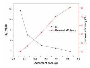
**Figure 10.** Effect of adsorbent dose on adsorption efficiency and capacity (V = 0.05 L, T = 25 °C, t = 240 min, pH = 6).
