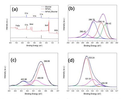
**Figure 5.** (**a**) X-ray photoelectron spectrometer plots of biochar, BiFeO<sub>3</sub>, and BiFeO<sub>3</sub>/biochar coupled magnetic material; high-resolution (**b**) C1s, (**c**) N1s, and (**d**) O1s spectra of BiFeO<sub>3</sub>/biochar coupled magnetic material.
