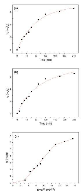
**Figure 14.** (**a**) Pseudo-first-order, (**b**) pseudo-second-order, and (**c**) intra-particle diffusion model curves for methylene blue adsorption onto BiFeO<sub>3</sub>/biochar coupled magnetic material.
