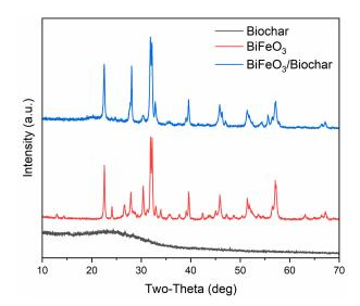
Figure 2. X-ray diffraction patterns of biochar, BiFeO<sub>3</sub>, and BiFeO<sub>3</sub>/biochar coupled magnetic material.
