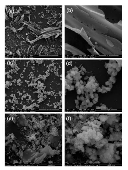
**Figure 3.** Scanning electron microscopy images of (**a**,**b**) biochar, (**c**,**d**) BiFeO<sub>3</sub>, and (**e**,**f**) BiFeO<sub>3</sub>/biochar coupled magnetic material.
