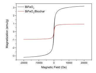
Figure 6. Magnetization curves of BiFeO<sub>3</sub> and BiFeO<sub>3</sub>/biochar coupled magnetic material.
