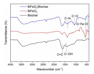
Figure 7. Fourier transform infrared spectra of biochar, BiFeO<sub>3</sub>, and BiFeO<sub>3</sub>/biochar magnetic material.
