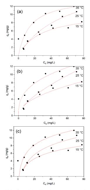
**Figure 13.** Isotherm model data for methylene blue adsorption onto BiFeO<sub>3</sub>/biochar coupled magnetic material: (**a**) Langmuir, (**b**) Freundlich, and (**c**) Temkin models.
