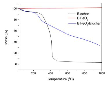
Figure 8. Thermogravimetric curves of biochar, BiFeO<sub>3</sub>, and BiFeO<sub>3</sub>/biochar coupled magnetic material.
