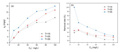
**Figure 11.** Effect of initial methylene blue concentration  $C_0$  and reaction temperature on (**a**) adsorption capacity and (**b**) removal efficiency (V = 0.05 L, pH = 6.0, t = 240 min, m = 0.1299 g).
