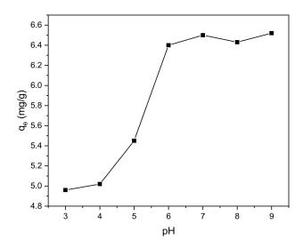
**Figure 9.** Effect of pH on the adsorption process (V = 0.05 L, T = 25 °C, t = 240 min, m = 0.1299 g).
