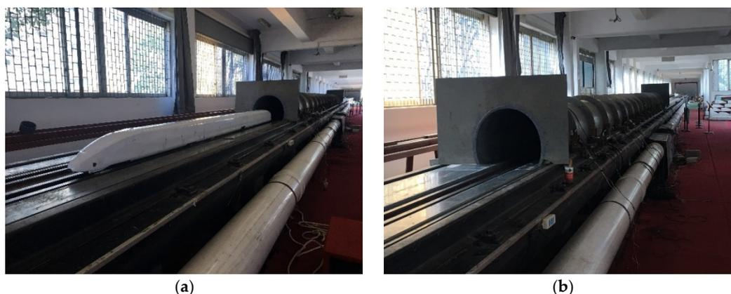
**Figure 2.** Moving model tests of aerodynamics in tunnels. (a) model train; (b) model tunnel.
