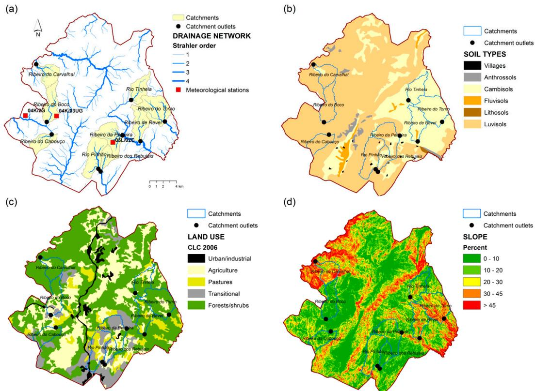
**Figure 8.** Geographic data used in the hydrologic simulations based on ArcSWAT. (a) Hydrographic and meteorological data; (b) Soil data; (c) Land use data; (d) Topographic data.
