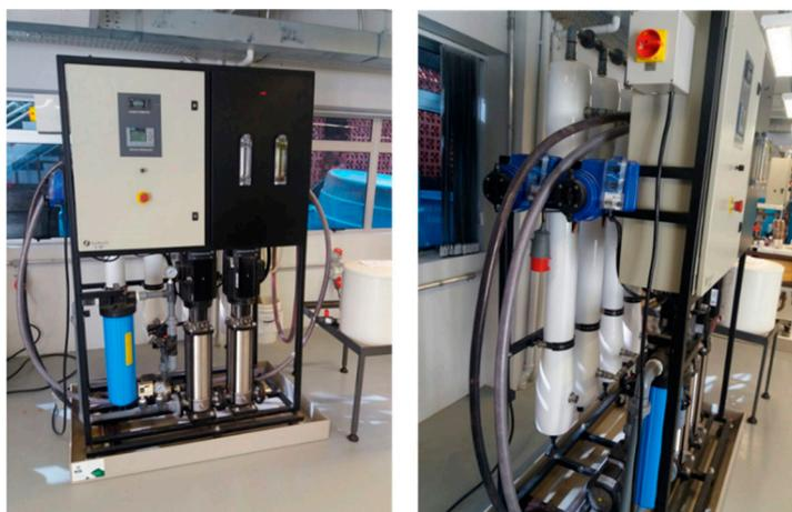
**Figure 1.** Reverse osmosis (RO) pilot system (PAM Selective Membranes, Rio de Janeiro, Brazil) equipped by a spiral polyamide membrane module BW 30 (4040) (Filmtec, Dow Chemical, Midland, MI, USA) with a membrane area of  $7.2 \text{ m}^2$ .
