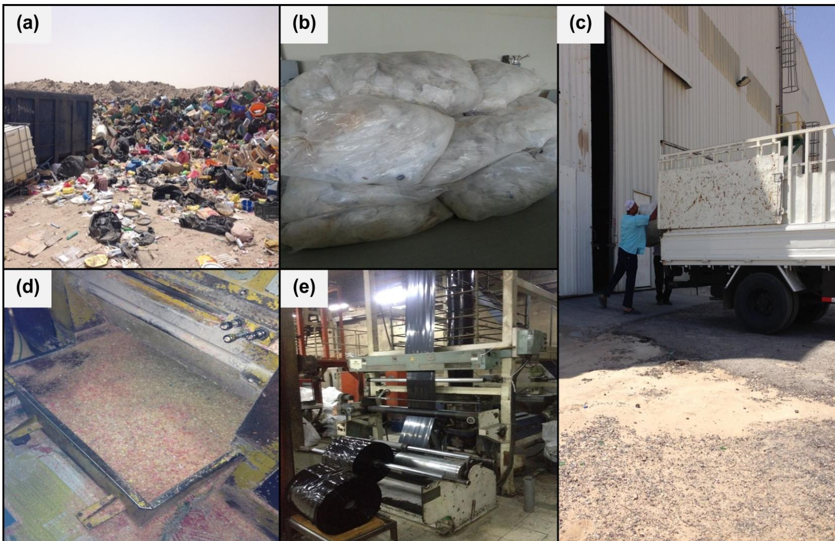
**Figure S1.** The various stages of the recycling procedure undertaken in this work showing (a) reclaimed plastic waste at landfill site, (b) storage of waste material, (c) transportation, (d) milling machine assembly, finally; (e) compounding of blends.
