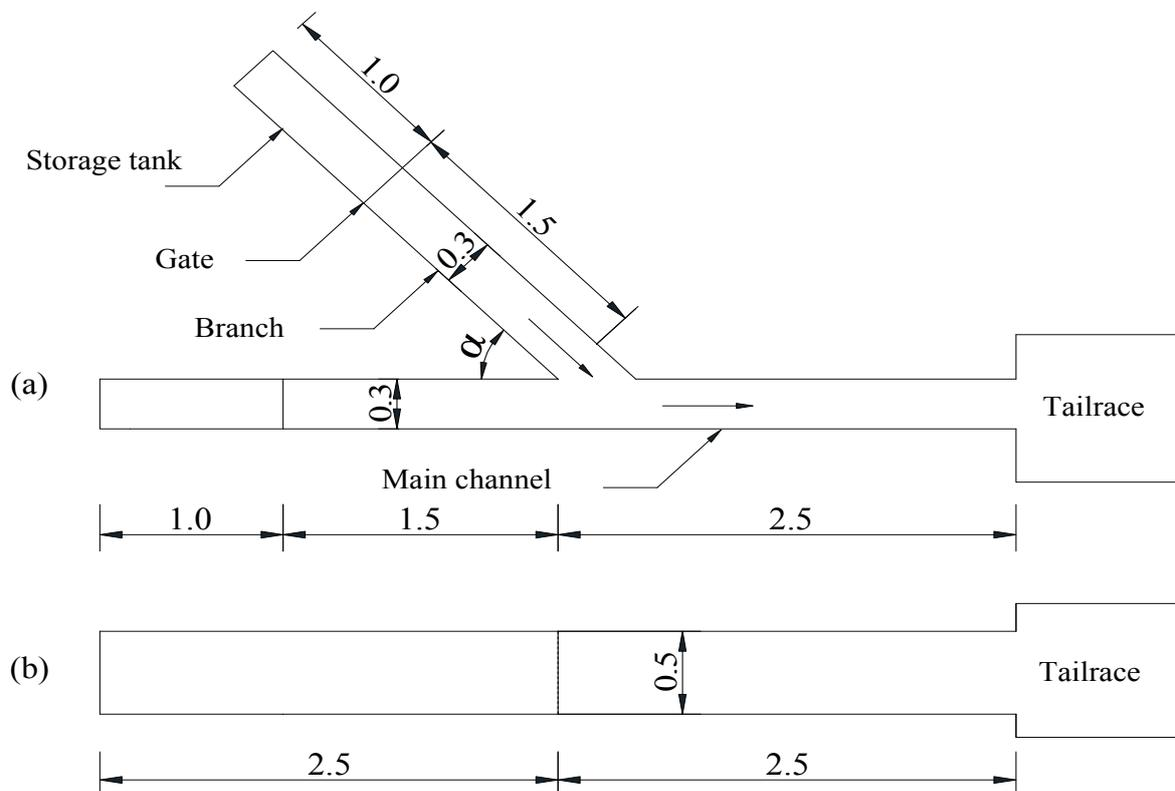
Figure 3. Sketch of the test channel, (a) plan view; (b) elevation (unit: m).
