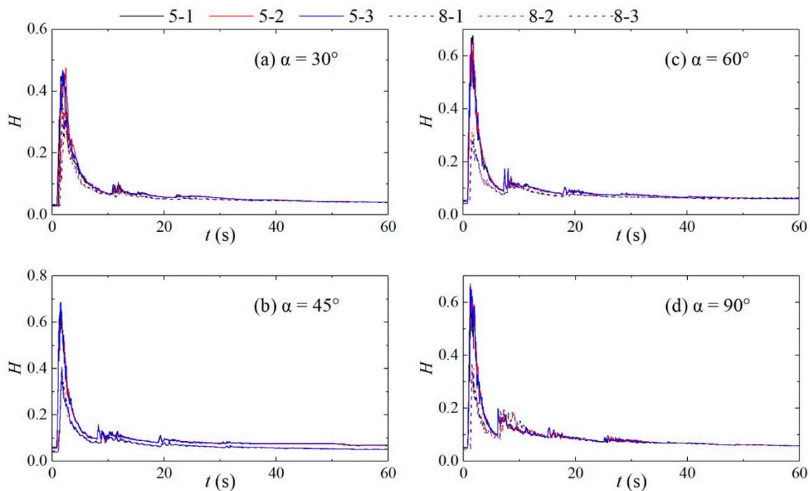
Figure 5. Variations in the water depth at measuring points #5 and #8. (a):  $\alpha = 30^\circ$ ; (b):  $\alpha = 45^\circ$ ; (c):  $\alpha = 60^\circ$ ; (d):  $\alpha = 90^\circ$ .
