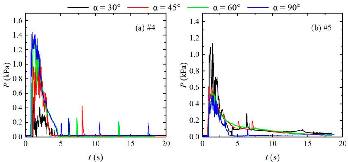
**Figure 13.** Pulsating pressure hydrographs at measuring points #4 and #5 of different configurations. (a): measuring points #4; (b): measuring points #5.
