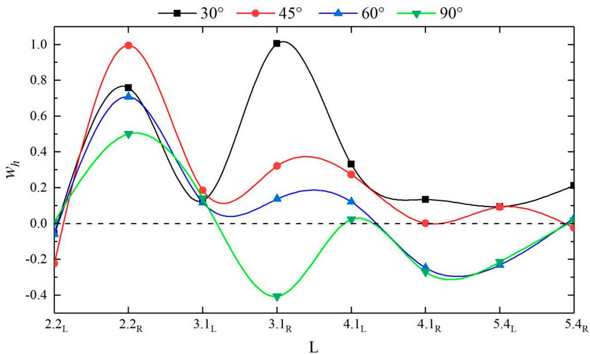
**Figure 10.**  $w_h$  values at each measuring point in the downstream straight sections of different configurations.
