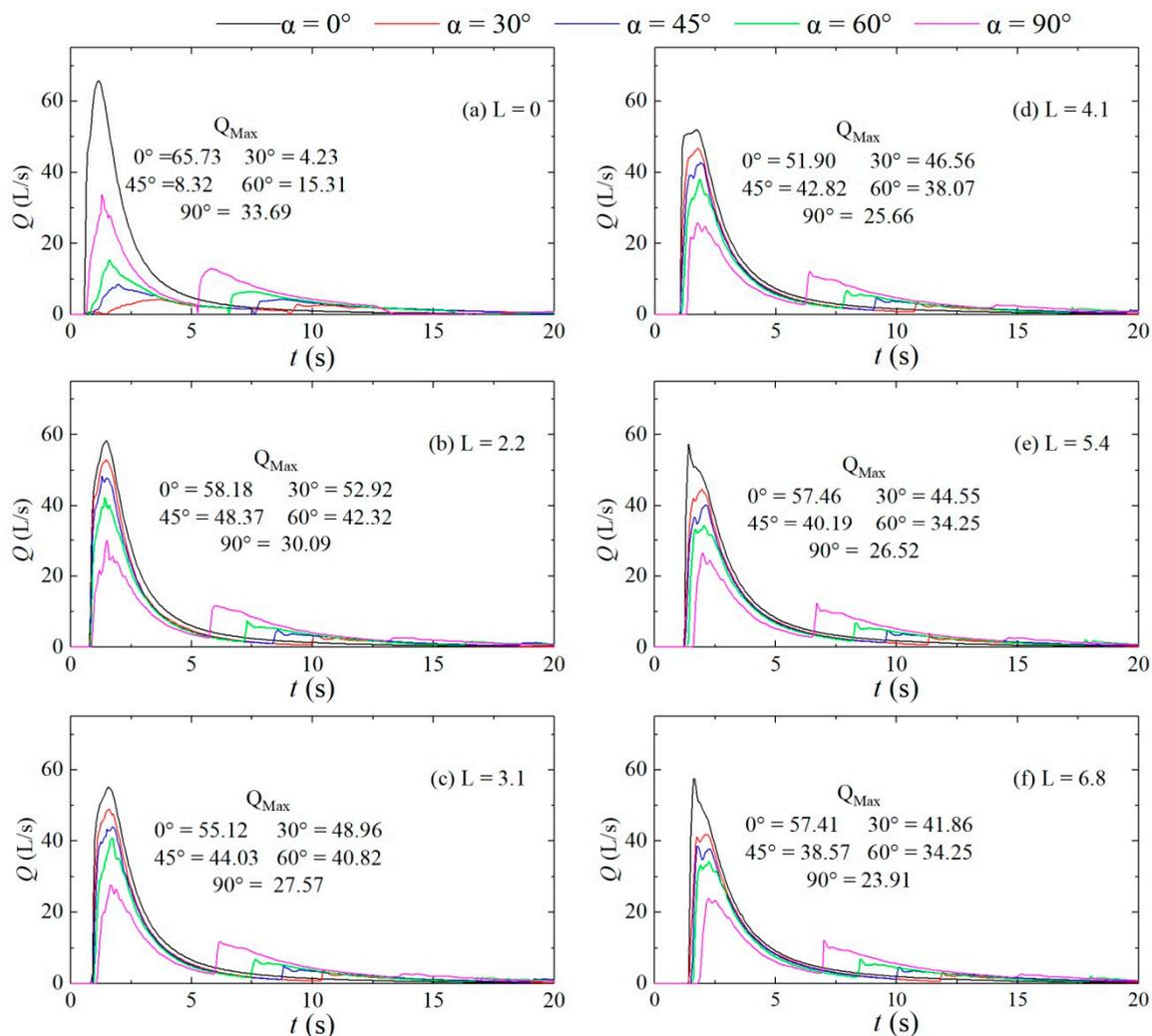
**Figure 17.** Flow discharge hydrographs for the downstream straight sections of different configurations. (a): L = 0; (b): L = 2.2; (c): L = 3.1; (d): L = 4.1; (e): L = 5.4; (f): L = 6.8.
