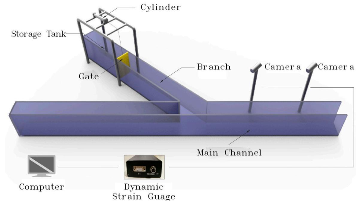
Figure 2. Sketch of the dam-break model test systems.
