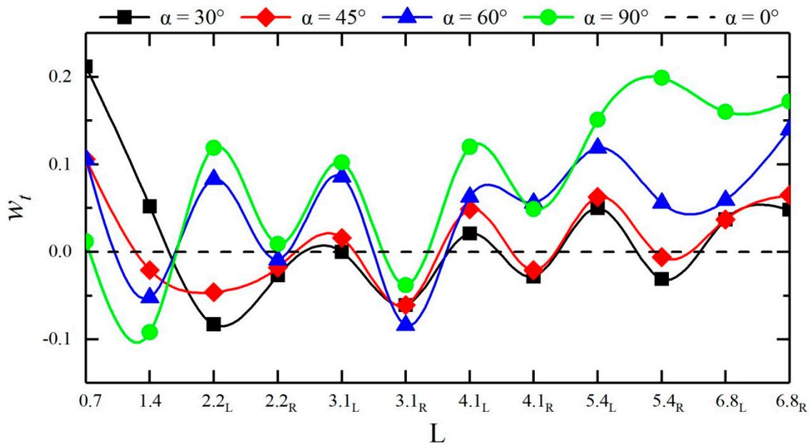
**Figure 12.** Rise time retardation factors  $w_t$  at each measuring point of different confluence configurations.
