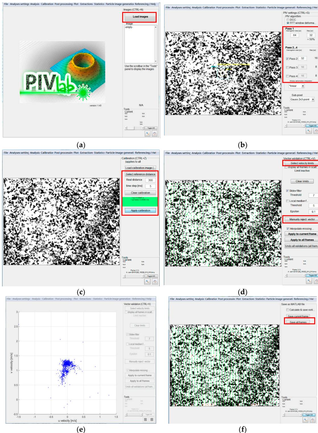
**Figure 14.** Procedure for particle image processing. (a) Image import; (b) window selection; (c) coordinate transformation; (d) local correction; (e) velocity range limit; (f) velocity vector output.
