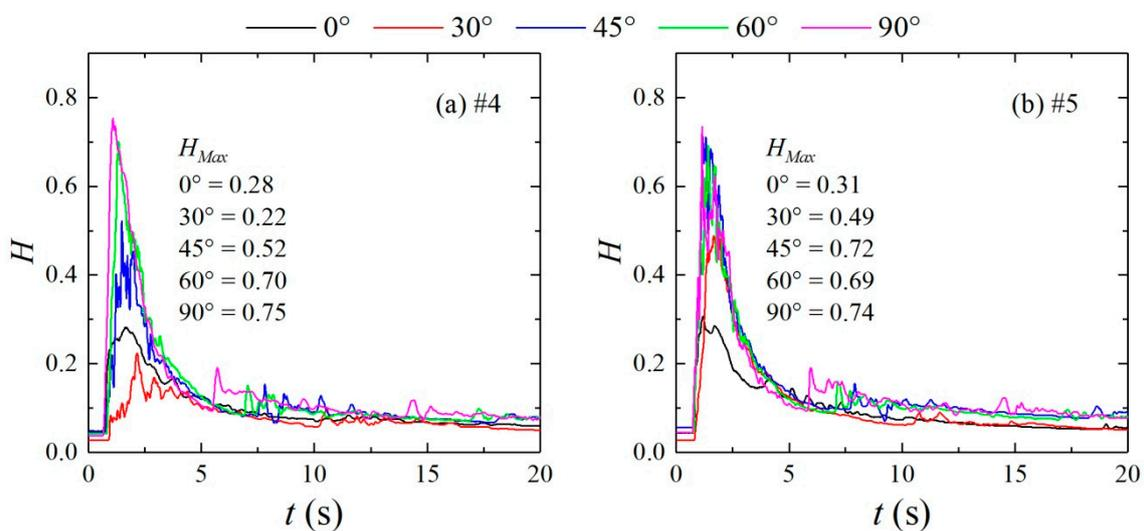
**Figure 7.** Variations in the water depths of different configurations at measuring points #4 and #5 over time. (a): measuring points #4; (b): measuring points #5.
