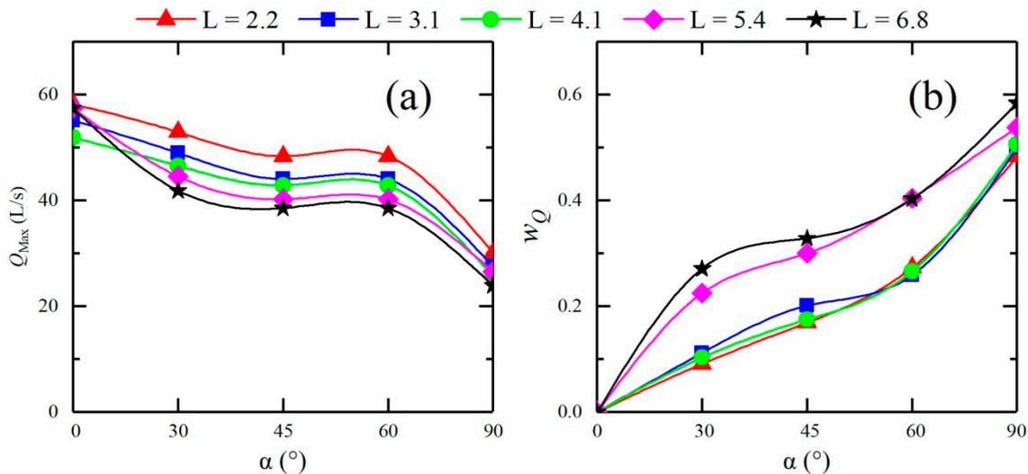
**Figure 18.** Peak flood discharge and discharge peak reduction factor at different cross-sections in the downstream straight sections of different configurations. (a): peak flood discharge; (b): discharge peak reduction factor.
