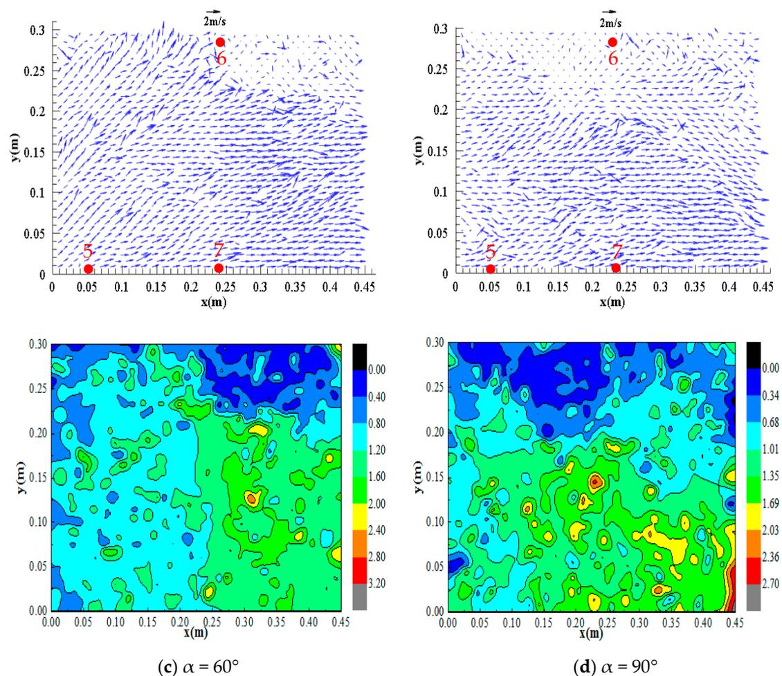
**Figure 16.** Distributions of the surface flow field of zone 2 under different configurations, (a)  $\alpha = 30^\circ$ ; (b)  $\alpha = 45^\circ$ ; (c)  $\alpha = 60^\circ$ ; (d)  $\alpha = 90^\circ$ .
