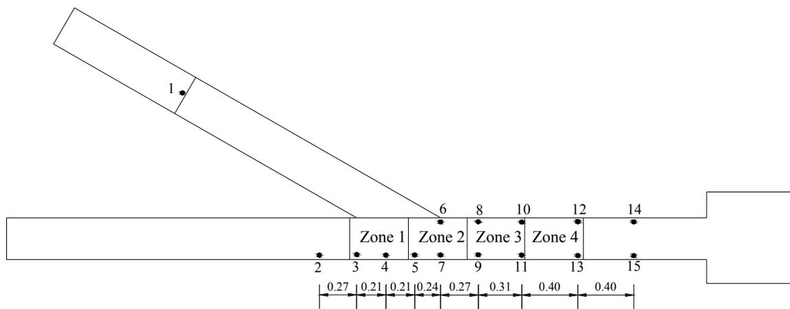
Figure 4. Layout of measuring points in the tests (unit: m).
