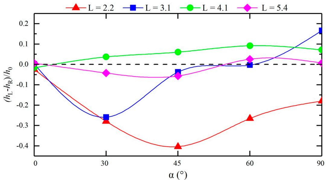
**Figure 9.** Comparison of the difference between the wave peaks at the left and right banks at each cross-section of the downstream straight section of each configuration.
