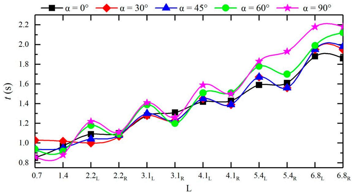
Figure 11. Water depth rise time  $t_j$  at each measuring point of different configurations.
