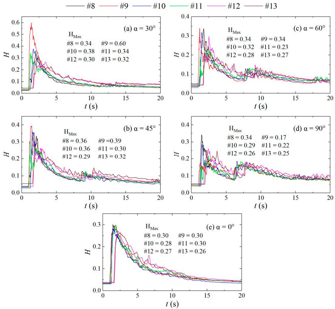
**Figure 8.** Variations in the water depths of the downstream straight sections of different configurations with time. (a):  $\alpha = 30^\circ$ ; (b):  $\alpha = 45^\circ$ ; (c):  $\alpha = 60^\circ$ ; (d):  $\alpha = 90^\circ$ ; (e):  $\alpha = 0^\circ$ .
