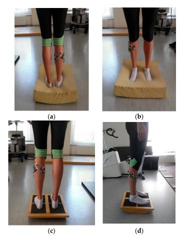
**Figure 1.** Illustration of EMG signal recording process. Note: the picture shows one of the young woman: (**a**) standing on a foam, plantar flexor of the foot gastrocnemius medialis (GM), gastrocnemius lateralis (GL), (**b**) standing on a foam, dorsal flexor of the foot tibialis anterior (TA), (**c**) standing on a "seesaw", plantar flexor of the foot gastrocnemius medialis (GM), gastrocnemius lateralis (GL), (**d**) standing on a "seesaw", plantar flexor of the foot peroneus longus (PER).
