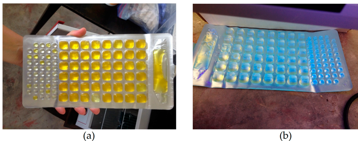
Figure 5. IDEXX Colilert-18 Quanti-Trays: (a) water sample testing positive for coliform; (b) water sample under UV light, testing positive for E. coli .
