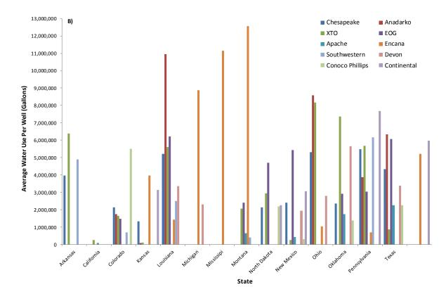
**Figure 1.** (**A**) Average Hydraulically Fractured Oil & Gas Well Water Demand Per Well across ten companies and six water stress environments and (**B**) fourteen US States and the aforementioned ten companies.
