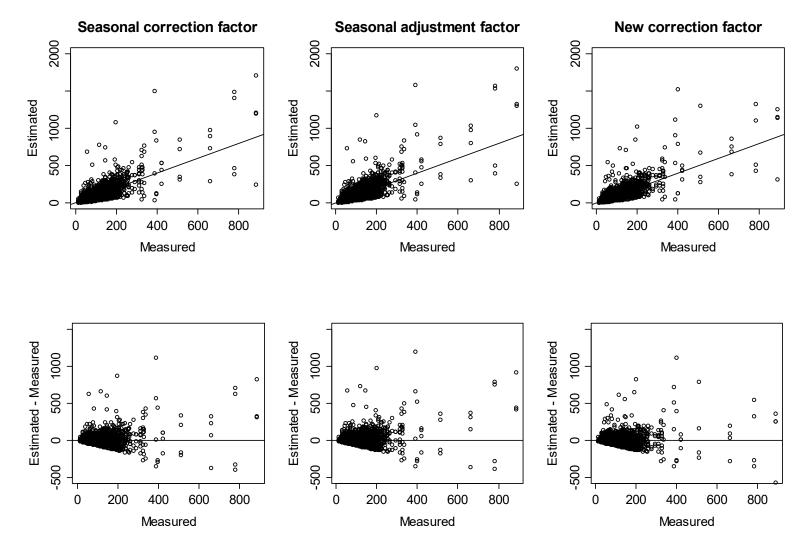
Figure 4. Comparisons of measured and estimated mean annual radon concentrations for detached houses.
