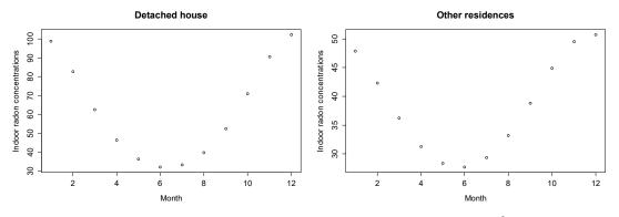
Figure 2. Monthly geometric mean of estimated indoor radon concentrations  $(Bq/m^3)$  calculated from Equation (7) for different types of houses.
