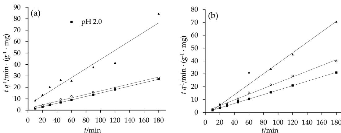
**Figure 6.** Pseudo second-order model for Cr(VI) removal by BFe<sup>0</sup>NPs (4%) at different pH values: (a) simulated wastewater; and (b) leachate wastewater.
