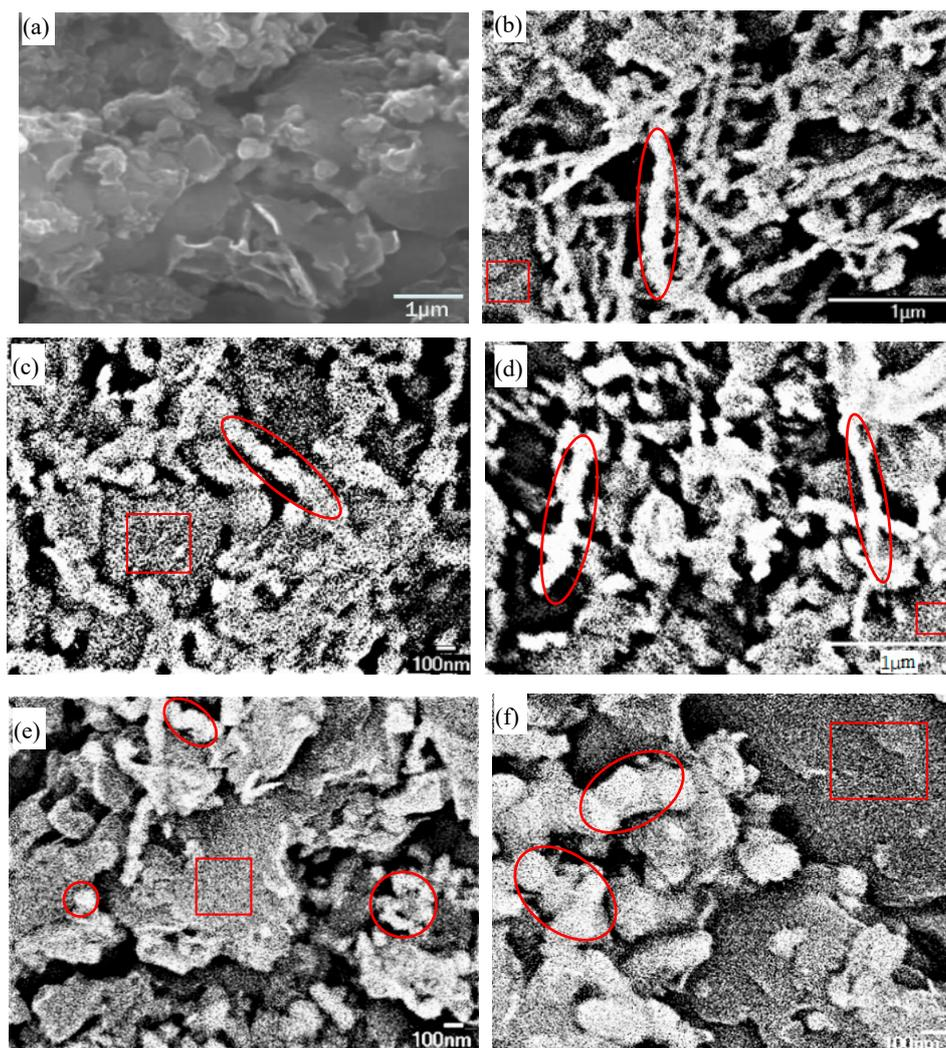
**Figure 1.** SEM images of bentonite (a) and BFe<sup>0</sup>NPs with different bentonite contents (b–f): (a) bentonite; (b) 1%; (c) 2%; (d) 3%; (e) 4%; and (f) 5%. The white chain-like conformations and dispersed particles represent Fe<sup>0</sup> (circles/ovals), and the grey backgrounds represent bentonite (rectangles).
