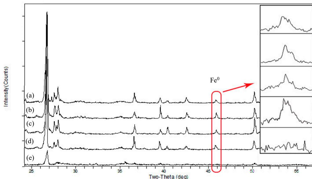
**Figure 2.** XRD characterization of BFe<sup>0</sup>NPs with different bentonite contents: (a) 1%; (b) 2%; (c) 3%; (d) 4%; and (e) 5%.
