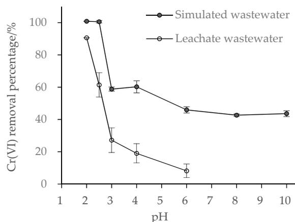
**Figure 3.** Effect of initial pH values on Cr(VI) removal ( $n = 3$ ) from wastewaters by BFe<sup>0</sup>NPs (4%).
