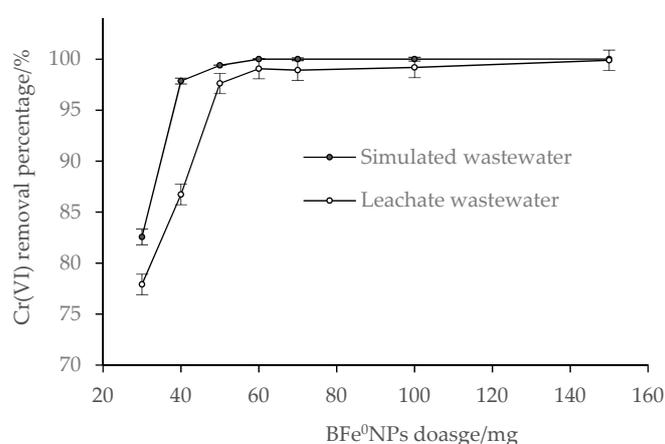
**Figure 5.** Effect of BFe<sup>0</sup>NPs (4%) dosage on Cr (VI) removal ( $n = 3$ ) from wastewaters.
