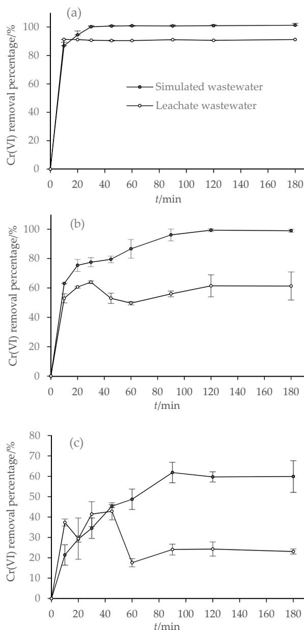
**Figure 4.** Effect of reaction time on Cr(VI) removal ( $n = 3$ ) from wastewaters by BFe<sup>0</sup>NPs (4%) at different pH values: (a) pH 2.0; (b) pH 2.5; and (c) pH 3.0.
