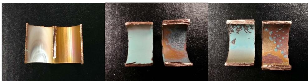
**Figure 7.** Cross-section of a copper pipe segment (**left**) after conditioning with tap water for 100 d, (**middle**) after 367 d orthophosphate addition and (**right**) after 433 d orthophosphate addition ceased.
