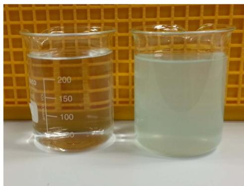
**Figure 6.** “Blue water” sample, before (right) and after filtration (left) with 0.45-micron pore-size nylon membrane.
