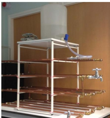
**Figure 1.** Photograph of the simulated lead-free premise plumbing system.
