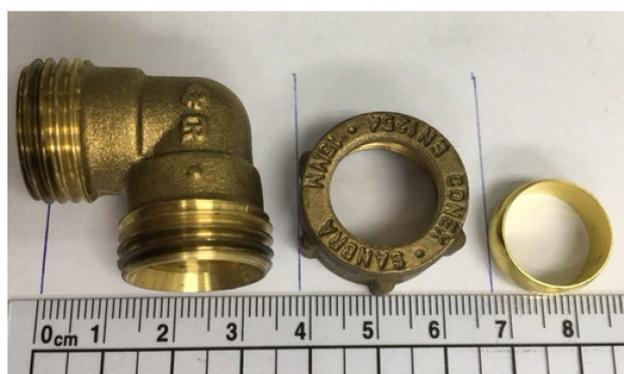
**Figure 2.** Photograph of brass fitting assembly: body (left); compression nut (middle) and compression ring (right).
