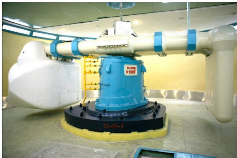
**Figure 12.** The centrifuge facility at IWHR.
