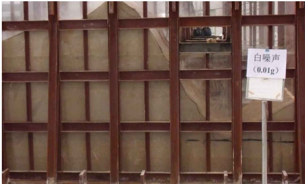
Figure 5. Shaking table test model of one-sided rock slope.
