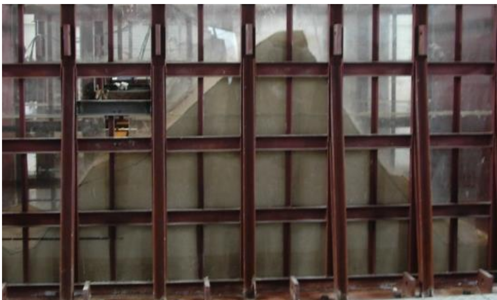
Figure 6. Shaking table test model of two-sided rock slope.
