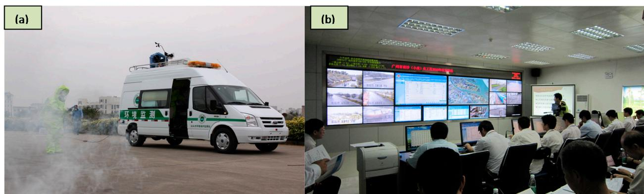
**Figure 11.** Photographs showing some parts of ERS: (a) the environmental monitoring car is used to detect the hazardous gas with toxic gas sensors; (b) accident commander is directing rescue operations in the emergency command center of XHCIP.
