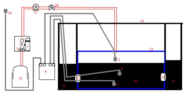
Figure 1. Designed layout of constructed balloon digester with the data acquisition system.
