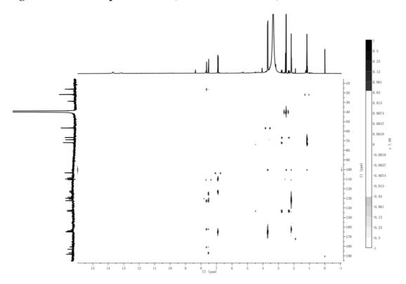
Figure S17. HMBC spectrum of 3 (500/125 MHz, DMSO-*d*<sub>6</sub>).
