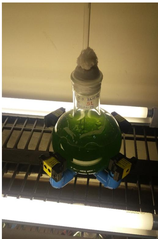
**Figure 6.** Photograph of the experimental setup for a single flask having the culture inside, surrounded by the permanent magnets, and under illumination.
