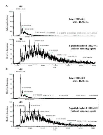
**Figure S1.** Electrospray ionization-mass spectrometry (ESI-MS) of intact HRL40-1 and HRL40-2 and their *S*-pyridylethylated derivatives in the absence of a reducing agent.
