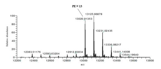
**Figure S2.** Electrospray ionization-mass spectrometry (ESI-MS) of *S*-pyridylethylated HRL40-2 in the presence of a reducing agent (tri-n-butylphosphine) (B).
