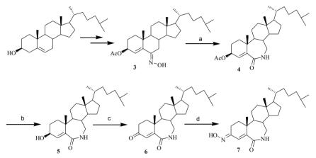
Reagents and conditions: (a)  $SOCl_2/THF$ , 0 °C; (b) 13%  $K_2CO_3/CH_3OH$ , stirred, 4 h; (c) Jones reagent/acetone, r. t., 2 h; (d)  $H_2NOH.HCl/Na_2Ac.3H_2O/EtOH$ , reflux.
