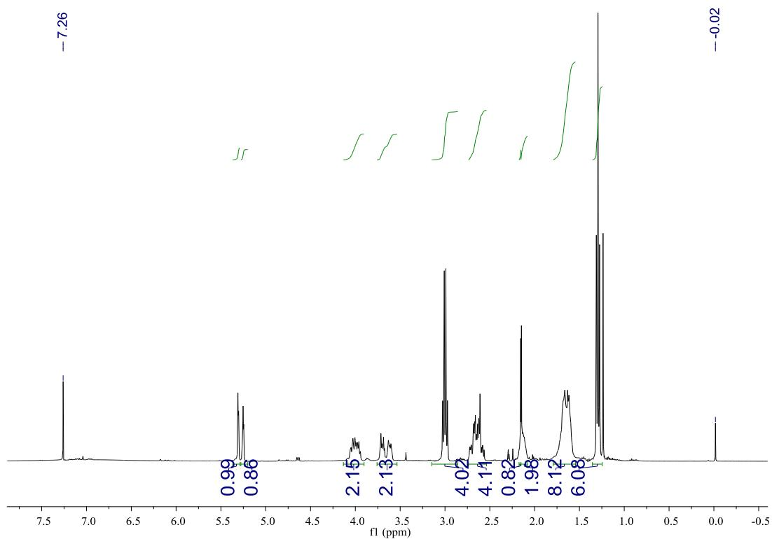
**Figure S33.**  $^1\text{H}$  NMR ( $\text{CDCl}_3$ , 400 MHz) of **9**.
