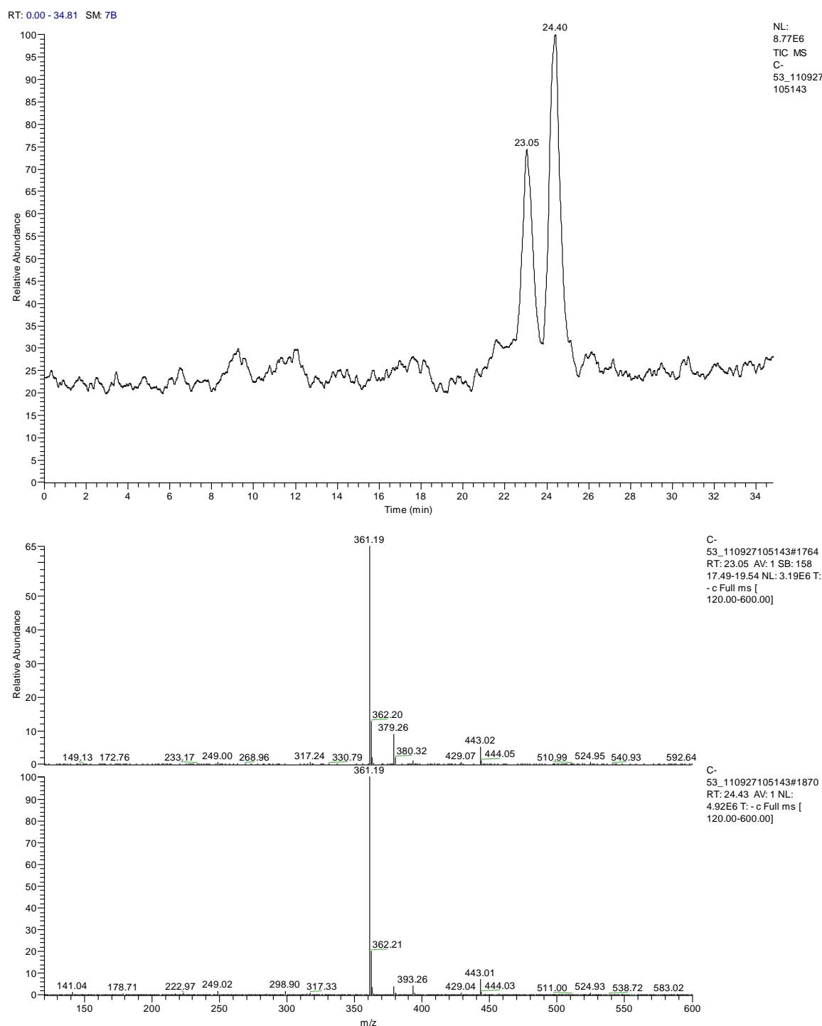
**Figure S47.** LC-MS of compound **23** using a gradient from 50% to 20% H<sub>2</sub>O over 60 min at 1 mL/min.
