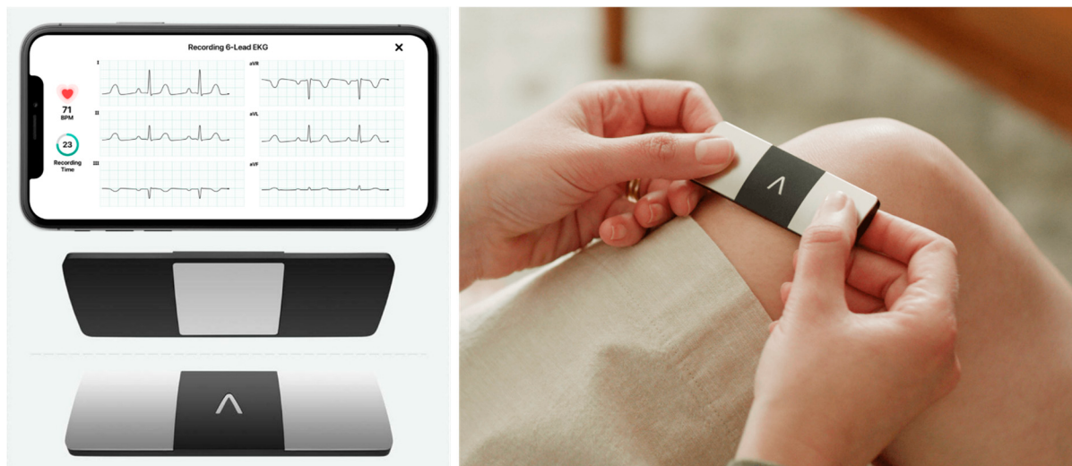
Figure 1. Handheld 6-lead ECG recording device in this study. The device is used with finger of right and left hand touching the respective electrode and a sample ECG rhythm is shown in a mobile phone display. Copyright with permission from Alivecor.
