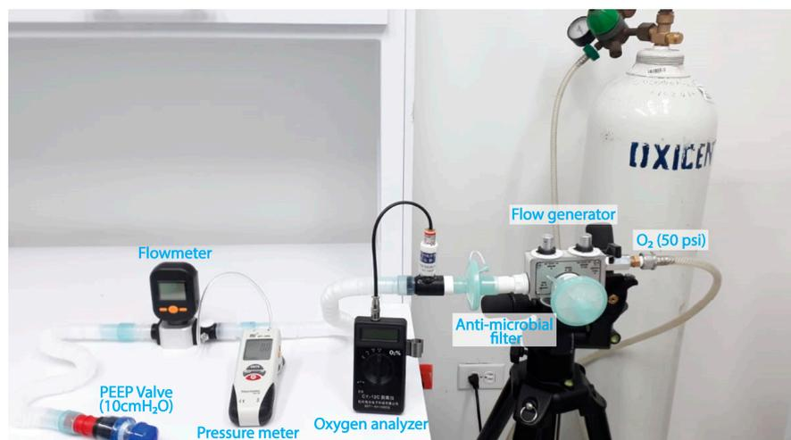
**Figure 2.** Configuration for validation of the CPAP-AirFlife™ flow generator.
