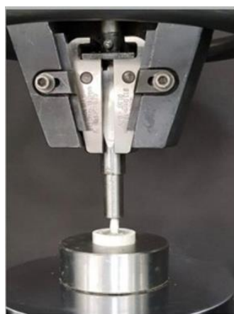
Figure 2. Fracture resistance test using Universal Testing Machine.
