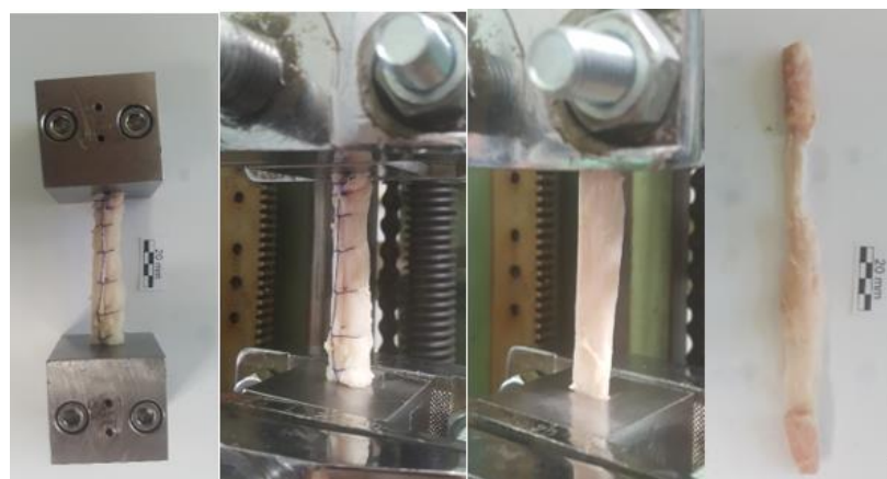
Figure 2. Graft preparation and testing on a mechanical testing machine.
