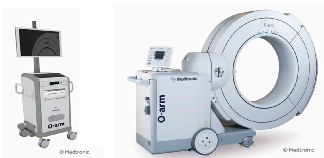
**Figure 1.** O-arm<sup>®</sup> and navigation device. The X-ray tube and flat-panel detector (FPD) rotate 360° inside the gantry, and three-dimensional (3D) scanning can be performed in approximately 13 s. High-precision 3D reconstruction is possible in a short amount of time.
