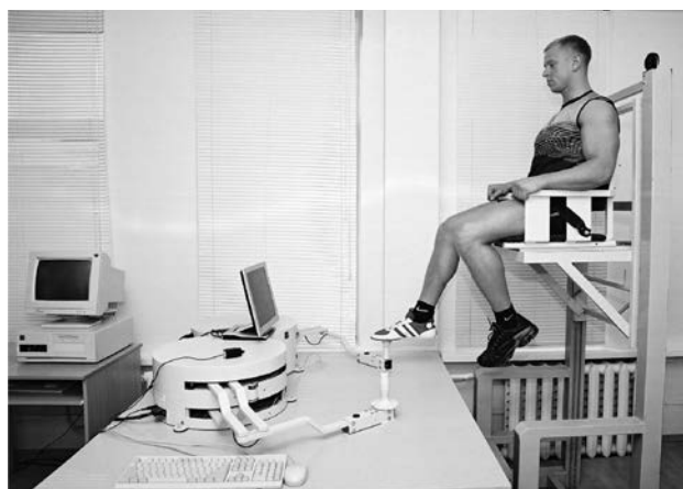
Fig. 1. DPA-1 equipment and subject position during the tests
