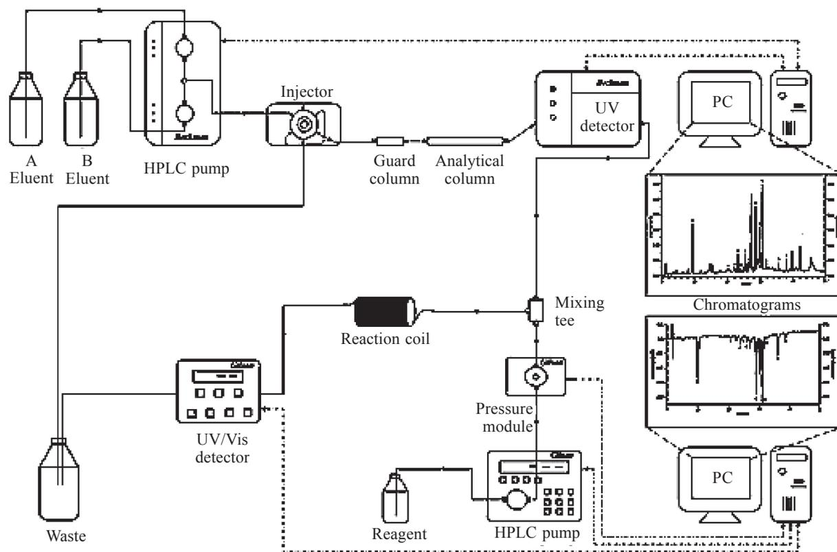
Fig. 1. HPLC-DPPH equipment system for analysis of individual antioxidants
