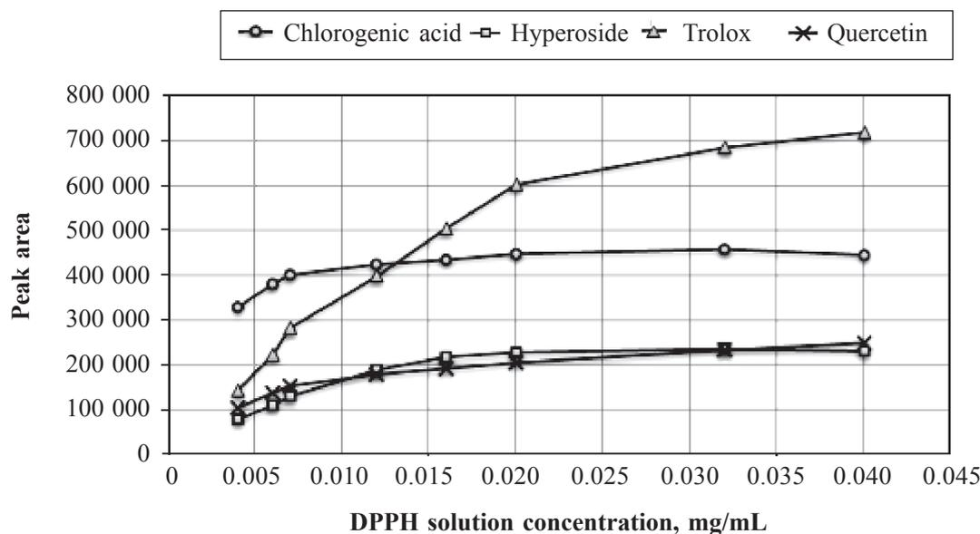
**Fig. 2. Dependence of standard peak area on DPPH solution concentration**
