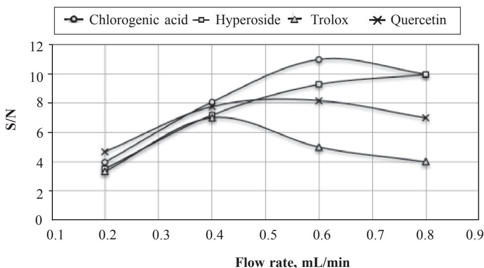
**Fig. 4. Dependence of peak height-to-baseline noise ratio (S/N) on DPPH solution flow rate**
