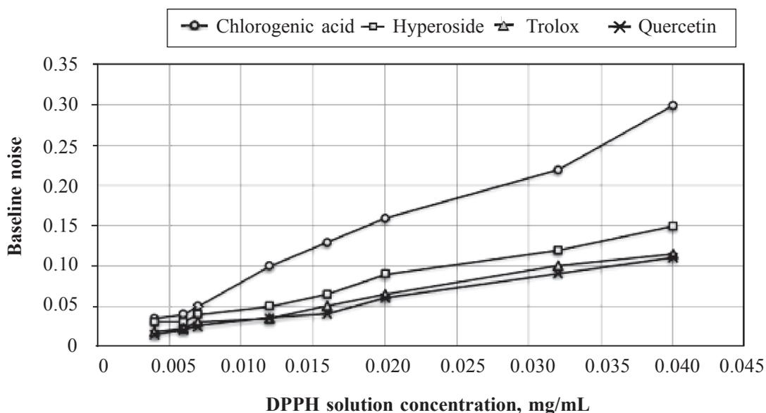
**Fig. 3. Dependence of baseline noise on DPPH solution concentration**
