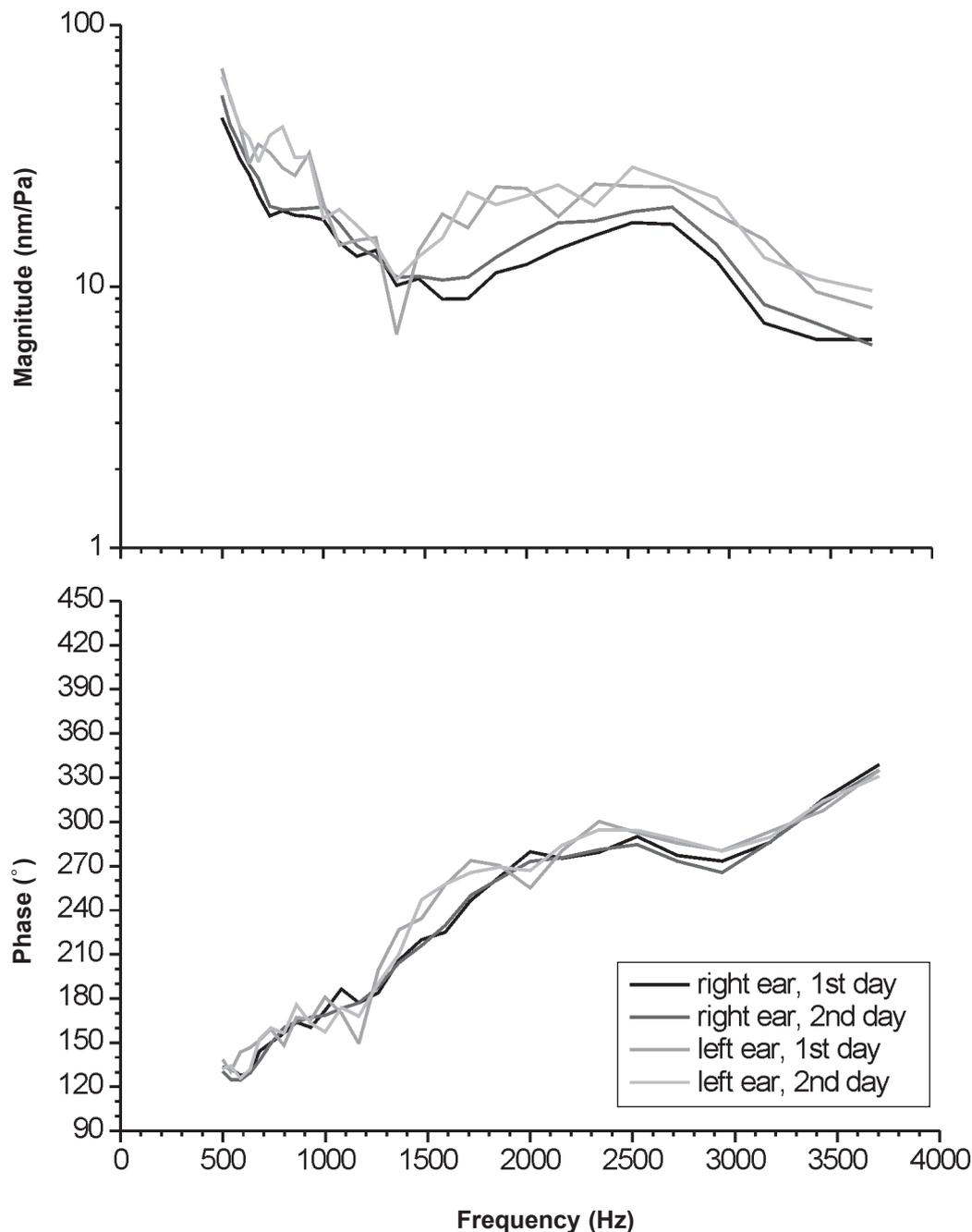
**Fig. 4.** Magnitudes and phases of laser Doppler vibrometry waveforms derived from point 1 of the tympanic membrane of the right and left ears in a representative test-subject at two consecutive days (1st day and 2nd day, respectively)
