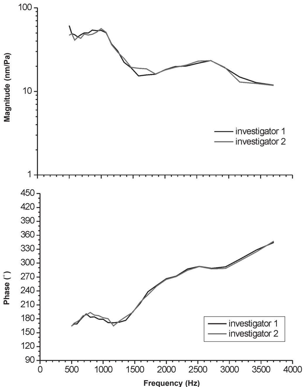
**Fig. 5.** Magnitudes and phases of laser Doppler vibrometry waveforms derived from point 1 of the tympanic membrane of the right ear in a representative test-subject by experienced and beginner investigators (1 and 2, respectively)
