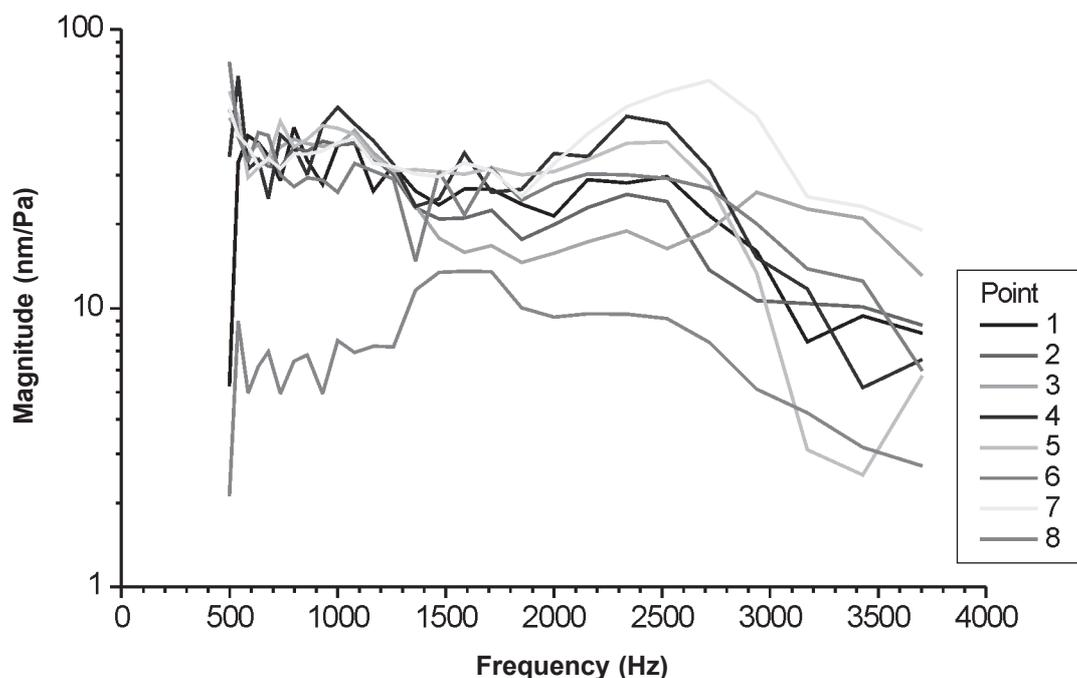
**Fig. 2. Magnitudes of laser Doppler vibrometry waveforms derived from different tympanic membrane loci (points 1–8) in a representative test-subject**
