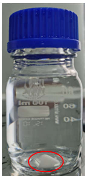
Figure 2. Morphology of the progesterone in situ gel after injection into release medium.
