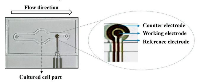
**Figure 11.** Photographic images of the electrode for measuring real-time ROS from cells exposed to drugs. A three-electrode system was adopted for electrodes based on the cyclic voltammetry method. The generated ROS oxidized working electrodes to induce electrical stimulation to measure the degree of ROS occurrence quantitatively.
