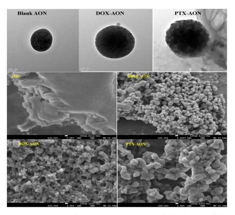
**Figure 1.** FE-TEM (**top**) and FE-SEM (**middle**, **bottom**) morphological images of blank AONs and drug-loaded AONs.
