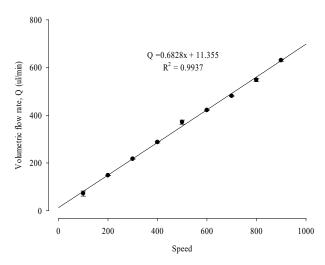
**Figure 10.** Standard calibration curve of a biomimetic microfluidic system between peristaltic pump speed and volumetric flow rate to determine the shear stress inside the sensor chip. The pump was operated for 1 min for each speed gauge, and the water weight delivered in the 1.5 microtubes was measured.
