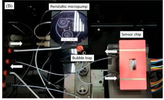
**Figure 9.** A schematic diagram of a biomimetic microfluidic system in which media circulate to simulate liver tissue and parts of the circulatory system. (**A**) Schematic diagram of the microfluidic components and the circulatory system and (**B**) photograph of a microfluidic system equipped with real-time generating ROS sensor chip ( $\rightarrow$  flow in,  $\leftarrow$  flow out).
