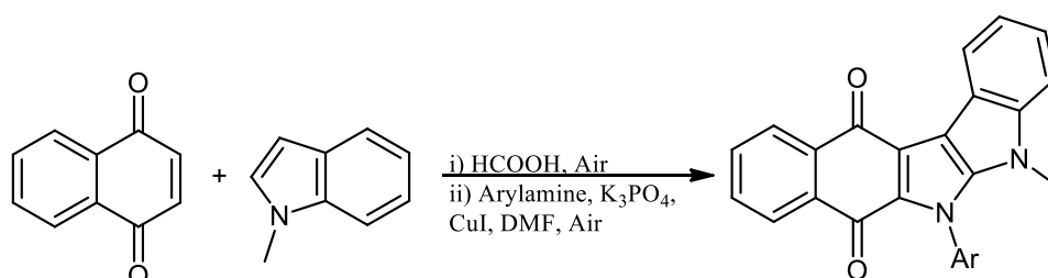
Figure 13. One-pot synthesis of indole-fused NQ derivatives.
