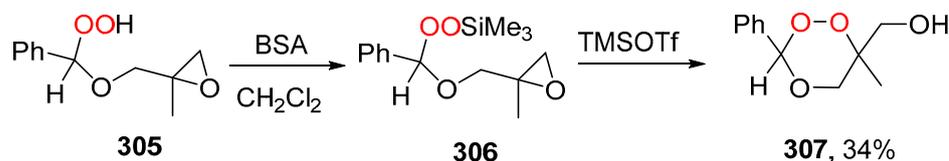
**Scheme 111.** Synthesis of substituted 1,2,4-trioxane **307**.
