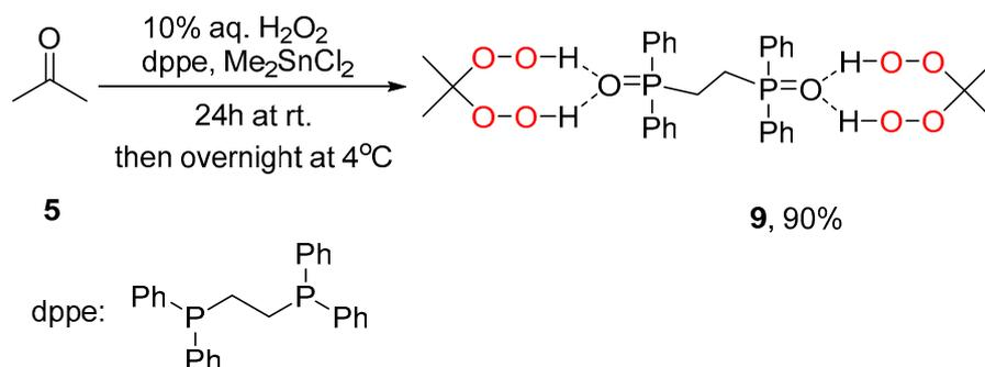
**Scheme 4.** Synthesis of (bis(diphenylphosphinoyl)ethane)·2(2,2-dihydroperoxypropane) 1:2 adduct **9**.
