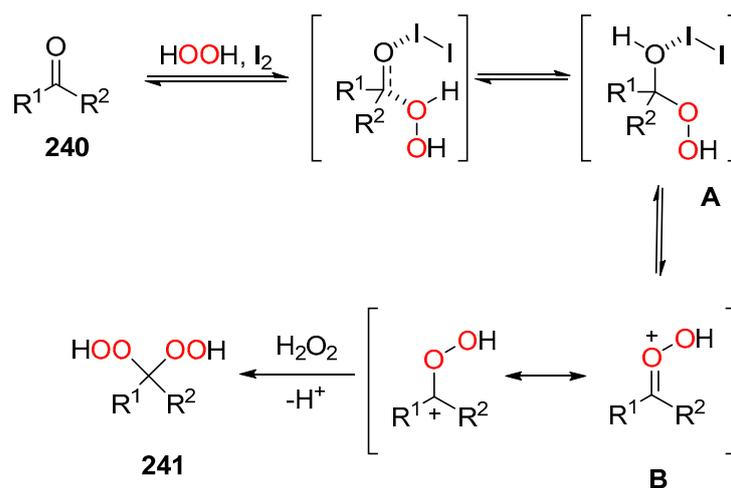
**Scheme 90.** The proposed mechanism for the assembly of geminal bisperoxide **241**.
