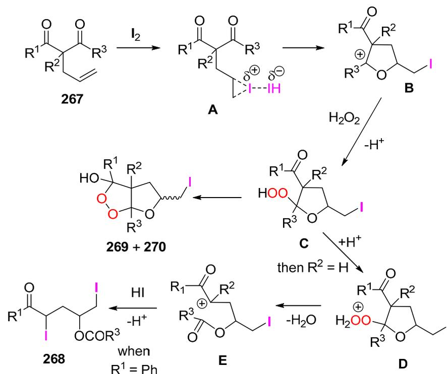
**Scheme 100.** The proposed mechanism for the assembly of bicyclic peroxides **269** and **270**.
