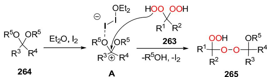
**Scheme 98.** The proposed mechanism for the assembly of 1-hydroperoxy-1'-alkoxyperoxides **265**.
