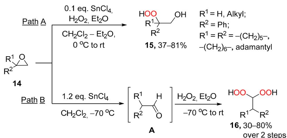
**Scheme 6.** Transformation of substituted oxiranes **14** into the corresponding  $\alpha$ -hydroxyhydroperoxides **15** and geminal 1,1-dihydroperoxides **16**.
