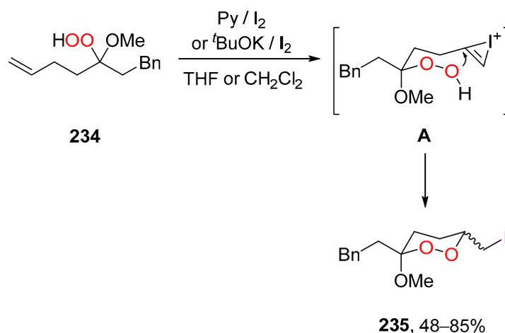
**Scheme 86.** Cyclization of unsaturated alkoxy hydroperoxide **234**.
