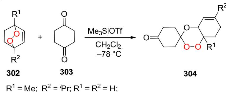
**Scheme 110.** Synthesis of substituted 1,2,4-trioxanes **304**.
