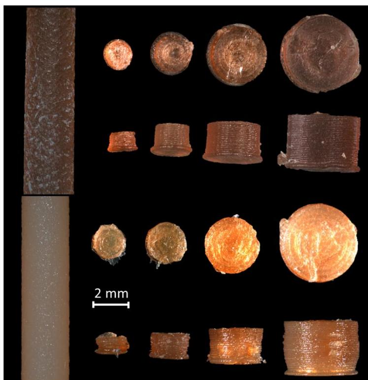
**Figure 1.** Microscopic images of the filaments and printed tablets with HPMC as polymer (top row: containing caffeine; bottom row: containing propranolol hydrochloride; from left to right: filament, mini tablet diameter 1.5, 2.0, 3.0, and 4.0 mm).
