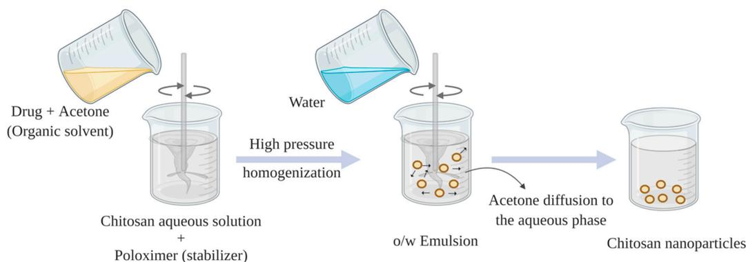
**Figure 7.** Schematic diagram of chitosan nanoparticles prepared via emulsion solvent diffusion.
