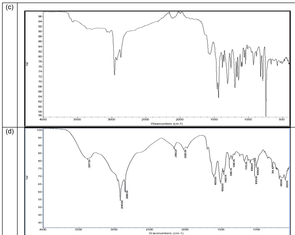
Figure SI-1. FTIR spectra of (a) Compound 1, (b) Compound 2, (c) PAA and (d) PAA-N. Spectra are averages of 64 scans.
